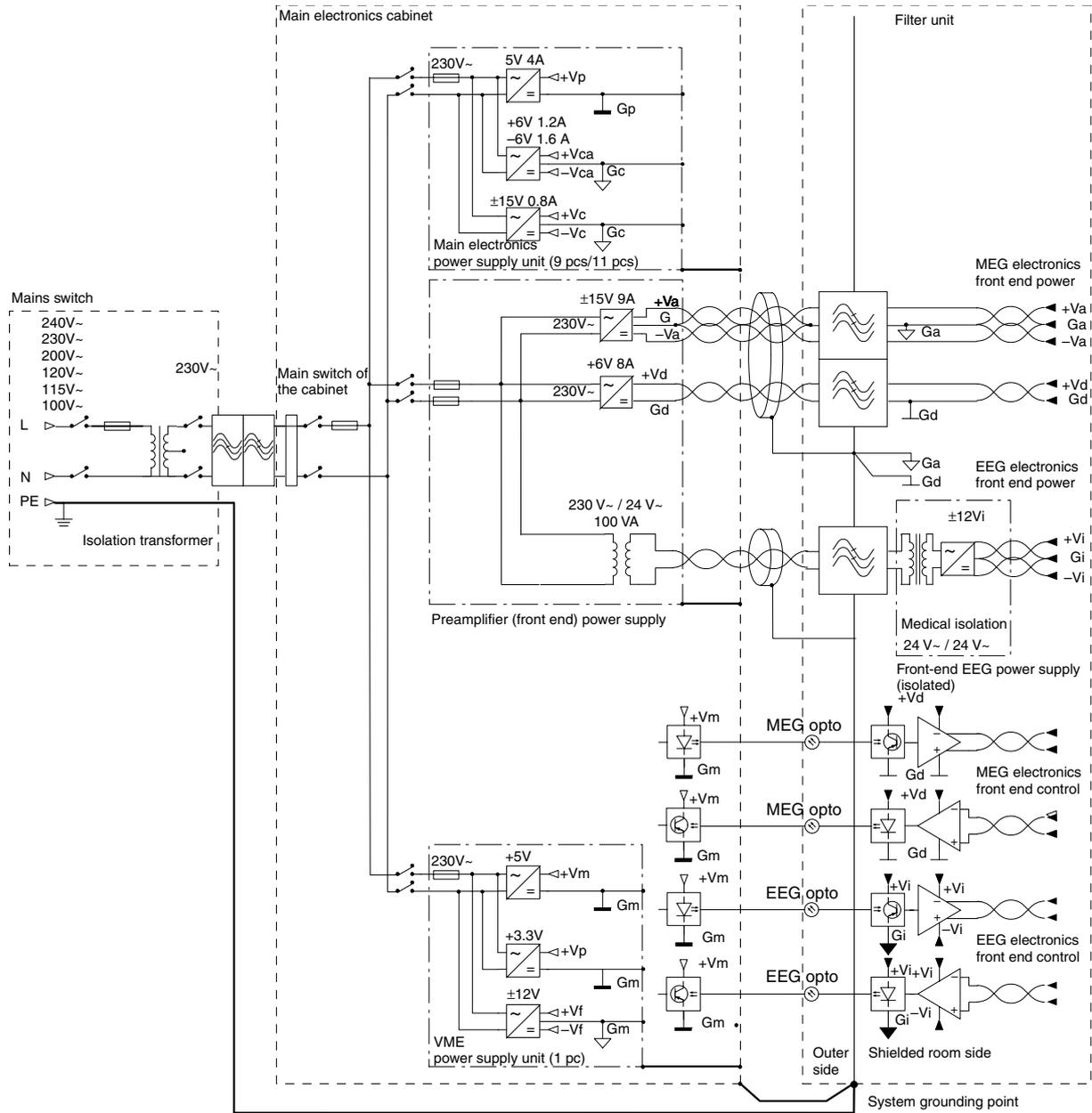
**Figure 3.10.** Schematic diagram of power supplies. NOTE: Stimulus system is not included.
