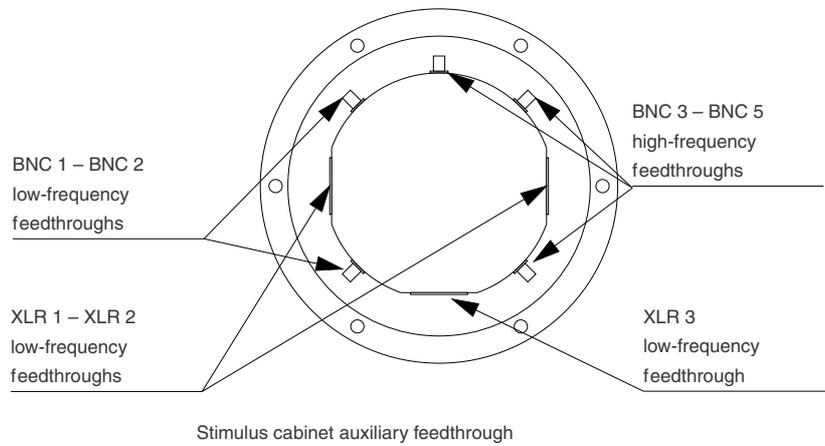
**Figure 3.9.a** Stimulus cabinet’s auxiliary signal feedthrough connectors. For specifications of the feedthrough filters, see 1.6.96.
