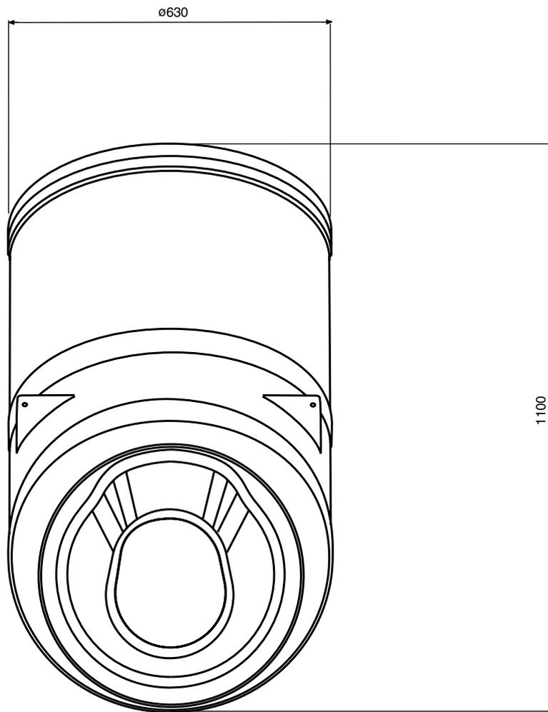
**Figure 2.2.** Dewar front view. Dimensions in millimeters.
