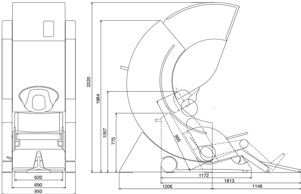
**Figure 2.3.** Gantry in upright measurement position. Dimensions in millimeters.
