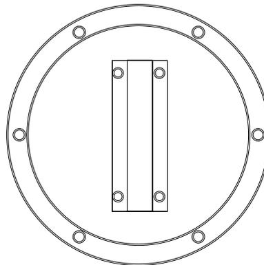
**Figure 3.9.b** Stimulus cabinet’s optional signal feedthrough connectors
