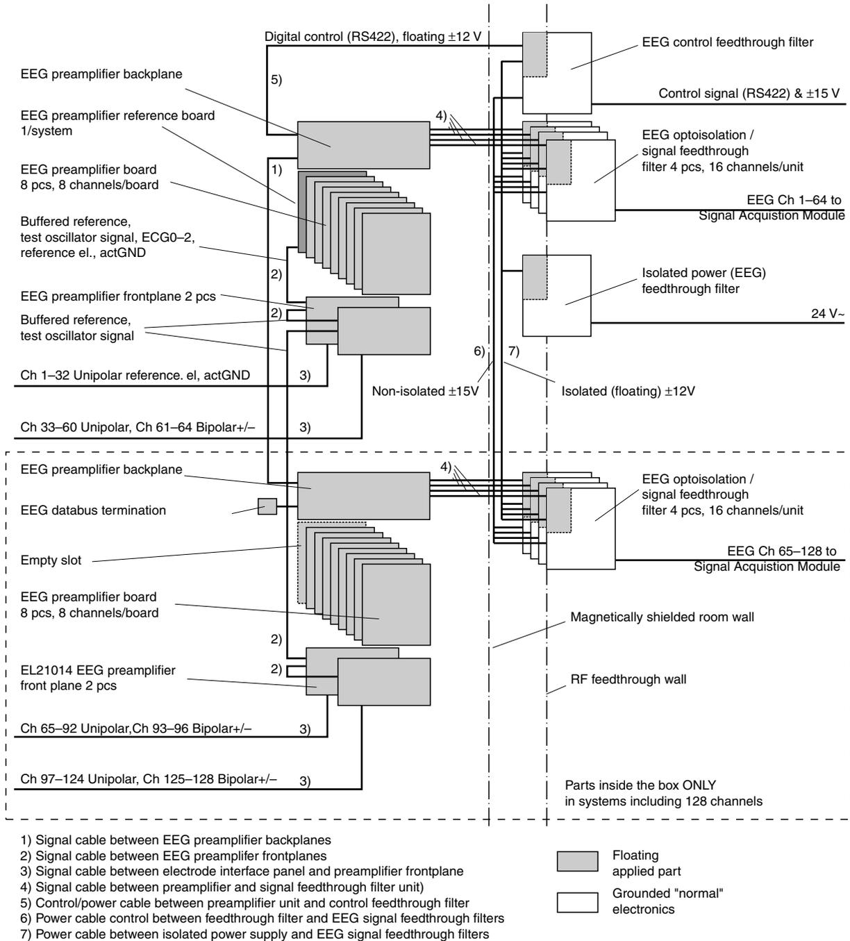
Figure 3.4. Block diagram of the EEG electronics
