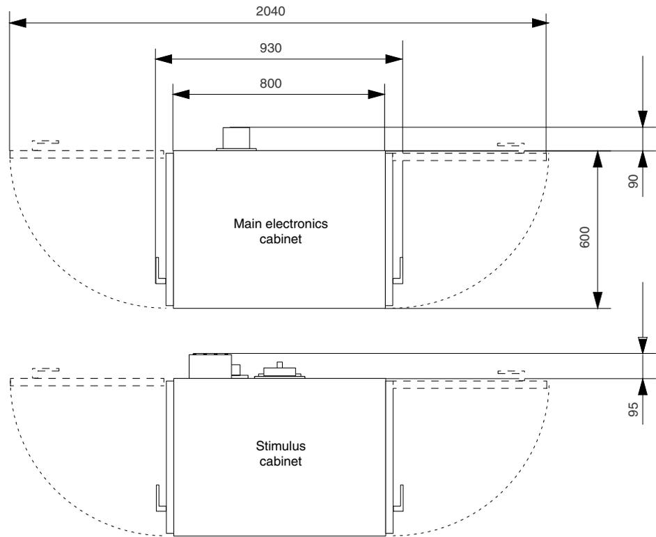
**Figure 2.5.** Electronics and stimulus cabinet dimensions (in millimeters).
