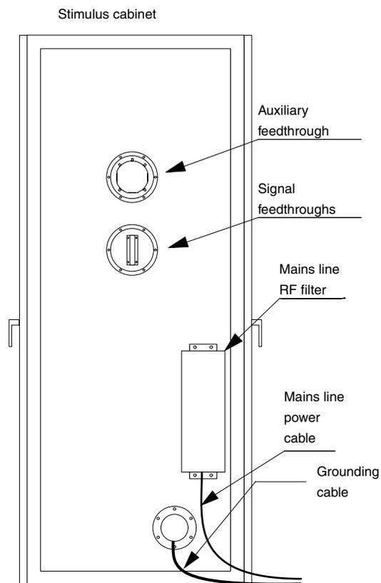
**Figure 3.8.** Stimulus cabinet, side view (side facing the magnetically shielded room)
