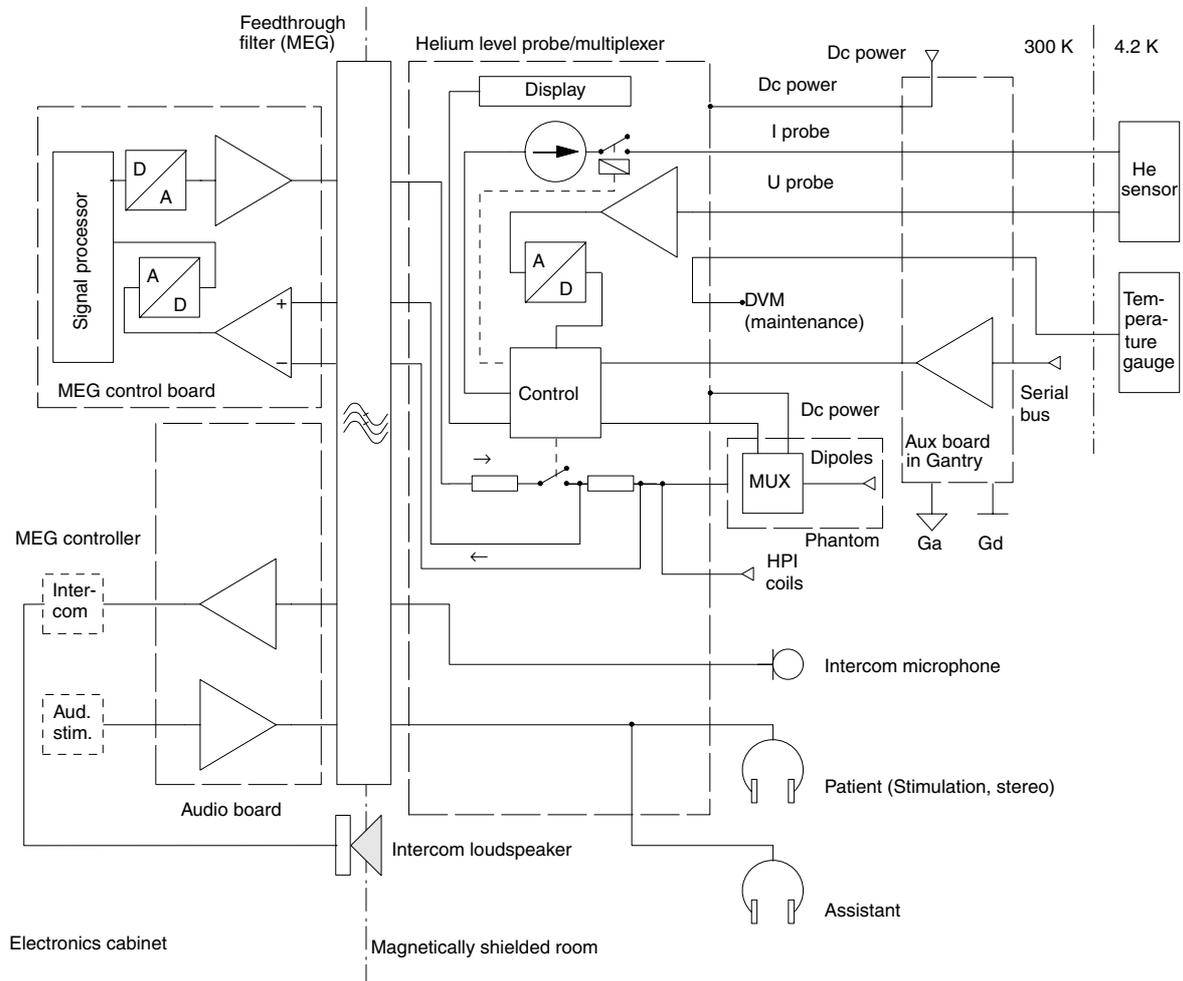
Figure 3.5. Schematic diagram of auxiliary electronics
