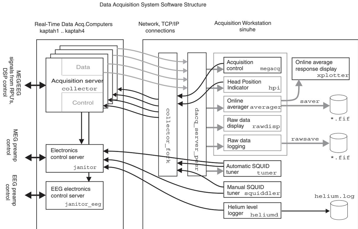
**Figure 3.15.** Data acquisition software block diagram
