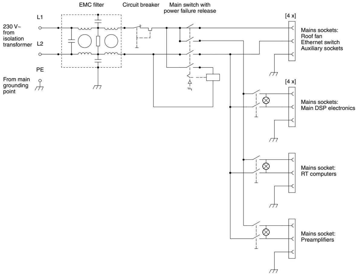
**Figure 3.7b.** Mains distribution in the main electronics cabinet
