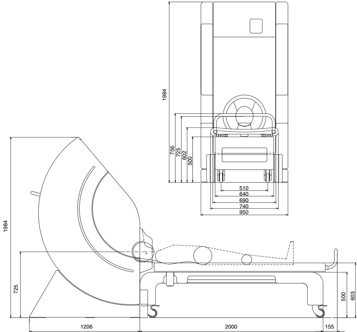
**Figure 2.4.** Gantry in supine position..Dimensions in millimeters.
