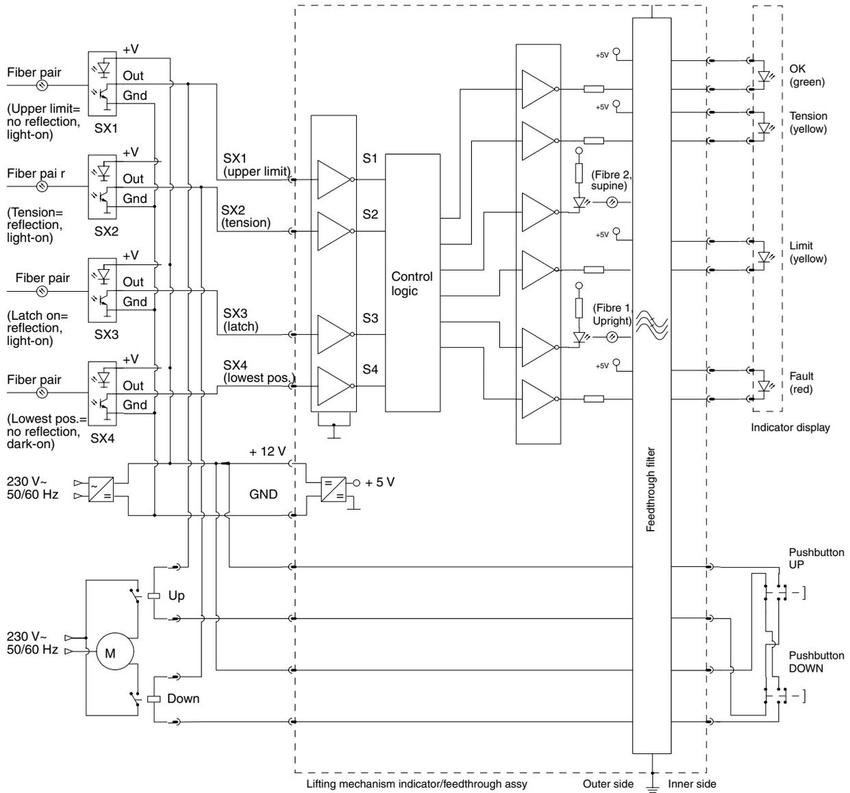
Figure 3.6. Schematic diagram of lifting mechanism electronics
