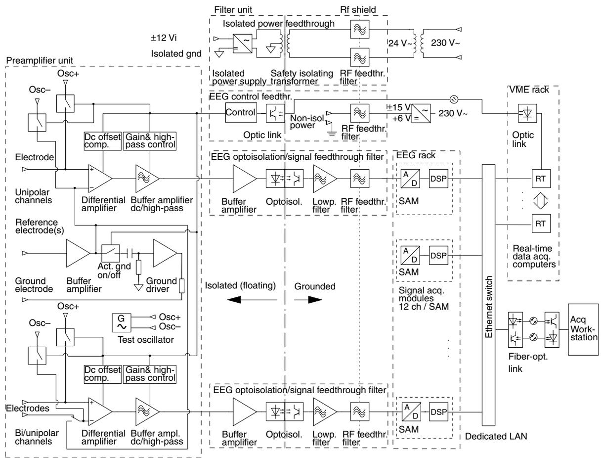
Figure 3.3. Schematic diagram of the EEG electronics
