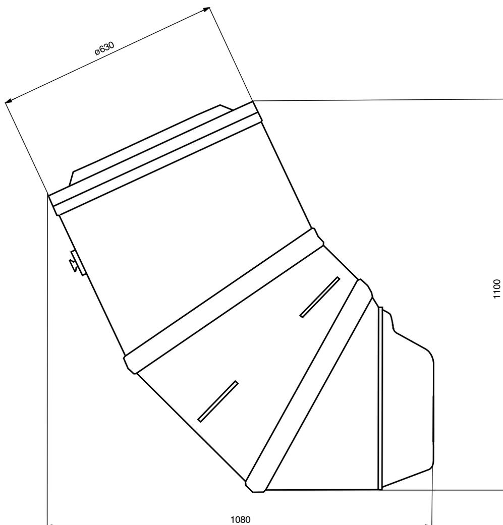
**Figure 2.1.** Dewar side view. Dimensions in millimeters.
