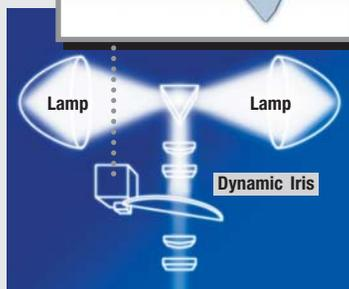
Incorporating Panasonic exclusive technology, the Dynamic Iris opens and closes with exceptional speed and precision as the input signal changes, resulting in accurate, real-time control of the light striking the DLP™ chips. The Dynamic Iris is posi-
