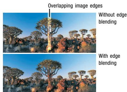
The built-in multi-screen processor enables enlarged multi-screen projection without using any additional special equipment. Colour matching and edge blending make it easier to obtain proper multi-screen picture quality.
