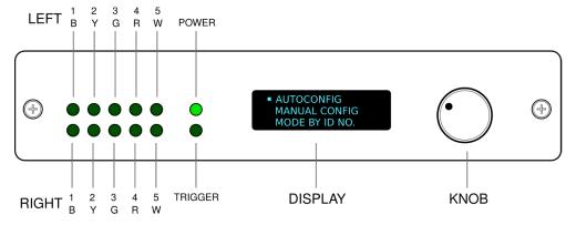
This drawing shows the front panel of the 932 with the indicator LEDs labeled as they would function in typical button box modes.
